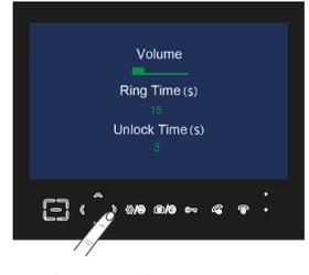
Press left & right to adjust the volume, the ring time (1-15 seconds) & unlock time (1-9 seconds).
